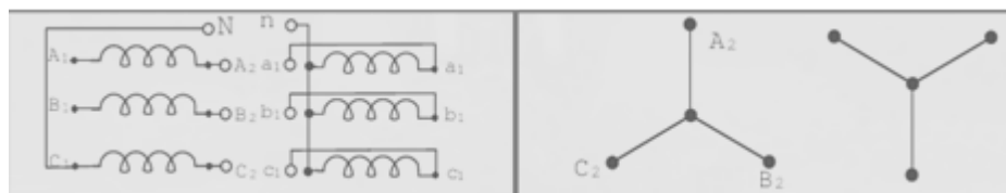
Fig 4.13. Yy6 connection and phasor diagram
